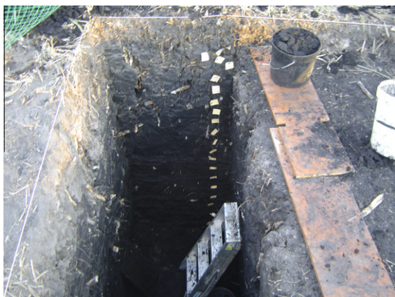
Fig. 7. The 4 m deep Pit B near the apex of the spring mound. The entire section consisted of peat. See Fig. 3 for location of the excavation.
